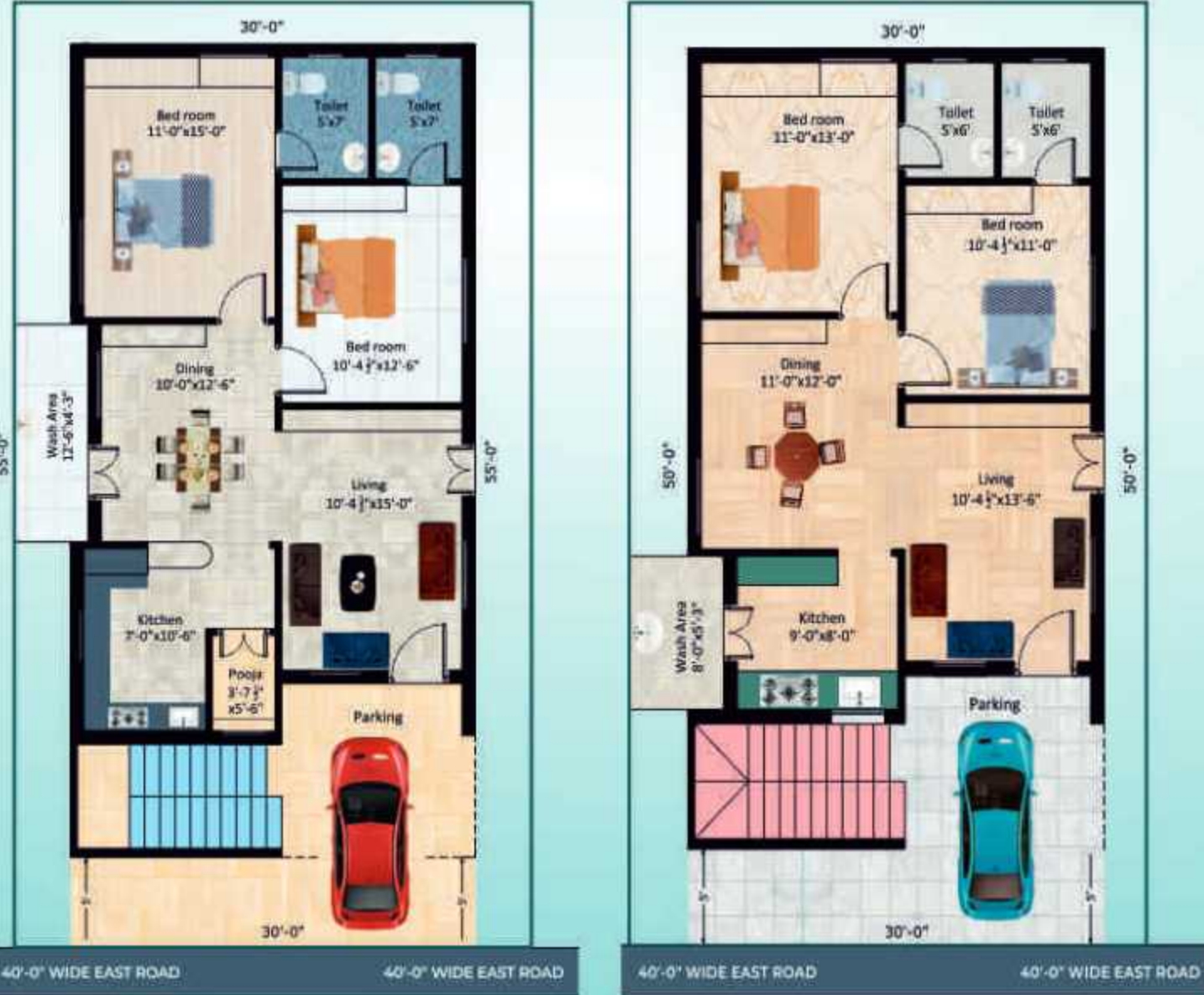
184 Sq. Yards GROUND FLOOR PLAN 1090.00 Sq. Fts Slab Area & 950.00 Sq. Fts Plinth Area
